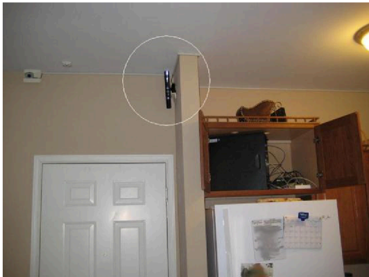
Figure 3 Kinect sensor installed in apartment with computer over the refrigerator
