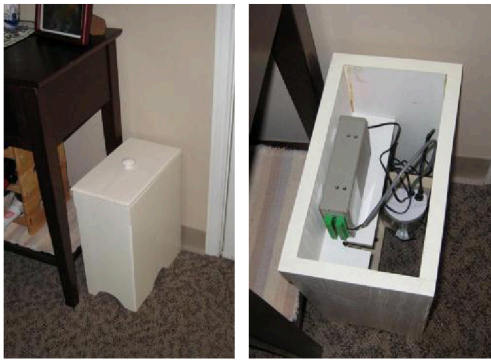
Figure 2 Radar unit in unobtrusive setting (left) Lid removed, showing data acquisition and radar (right)
