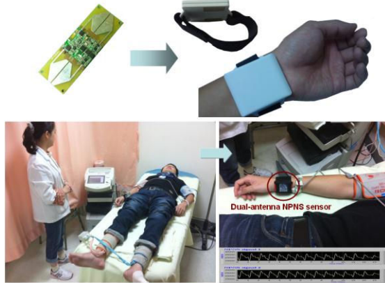
Fig. 6 The proposed NPNS based dual-antenna pulse signal detection device and clinical test scenario
