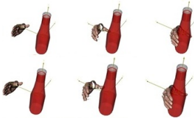
Fig. 9. On the top figure snapshots of the trajectory conducted by the human during grasping a bottle are depicted. On the bottom figure snapshots of the simulated hand following the trajectory generated by the proposed control law during grasping a bottle are depicted. In this figure the side view of the grasping experiments is depicted.
