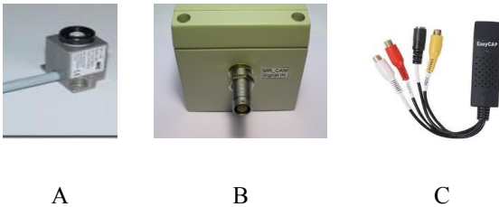
Figure 3 the MR Camera consists of three parts: A) Camera, B) Filter box, C) Video grabber
