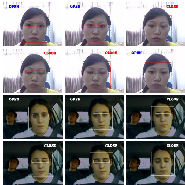
Figure 8. Output of the driver alertness monitoring system with two video sequences.
