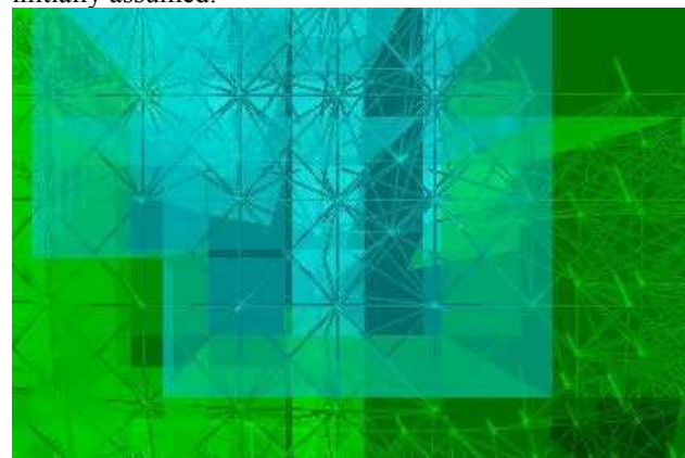
Figure 1. Electric grid embedded on the geometry. Two adjacent bundles are shown. Transparency is used to enhance visualization.
