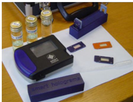
Figure 3: Smart Holograms prototype Hologram reader with integrated Bluetooth® connectivity.
