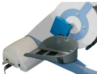
Figure 1: The strain gauge wireless acquisition device is inside the blue box, mounted on the left crank.
