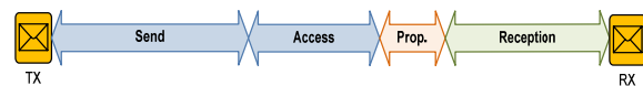
Figure 4: Times on sending, accessing, propagating and receiving reference messages. Propagation time is negligible versus send, access or reception times.
