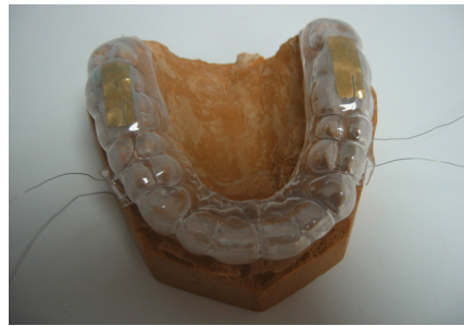
Figure 8: Splint with piezoelectric sensors for diagnosing bruxism.
