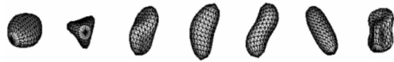
Figure 2: Graphical representation of seven low frequency vibration modes for surface model of ellipsoid (Syn and Prager, 1994).
