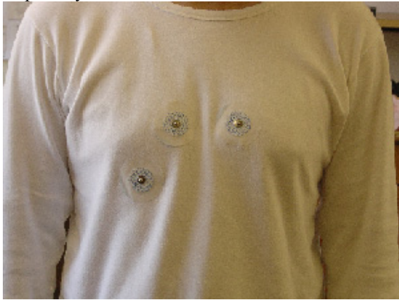
Figure 6: A photo of the patient wearing a electronic shirt ready to plug the RF modules.
