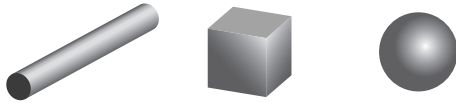
Figure 1: Long cylinder, cube and sphere of same volume ( V = 1000 ) have different surface ( S_{\text{cylinder}} = 694 (for this arbitrary proportion), S_{\text{cube}} = 600 , S_{\text{sphere}} = 484 ).
