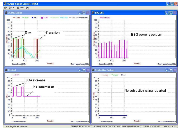
Figure 7: Screenshot of a tentative system operation. Top-left: aCAMS performance; top-right: psychophysiological response; bottom-left: LOA allocation; bottom-right: subjective ratings; status bar: monitoring of the system communication.
