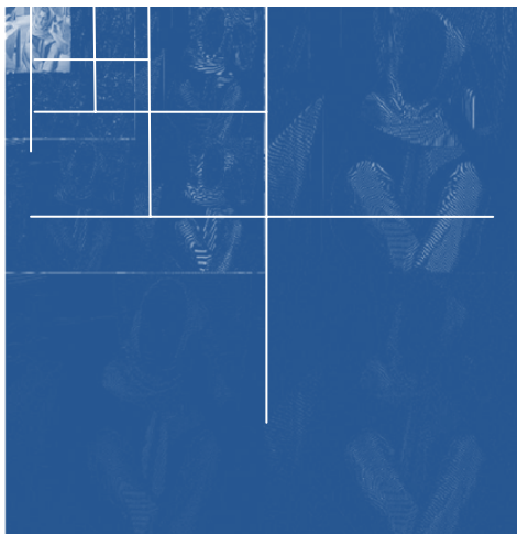
Figure 6: 3-level 2D-DWT using lifting scheme with Barbara image 512x512 pixels.
