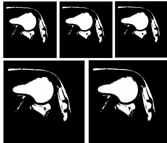
Figure 4: Slice 2. Segmentation image for one phase (2 classes) with: a) k-means b) Density mixture c) Active contours without edges d) Otsu's and e) Ridler Calvard algorithms.
