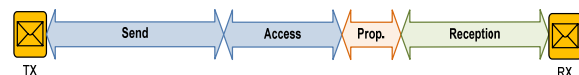
Figure 4: Times on sending, accessing, propagating and receiving reference messages. Propagation time is negligible versus send, access or reception times.
