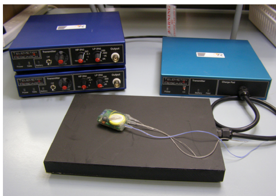
Figure 2: Wireless charger (right rear) and charging pad (foreground), implantable telemeter (on charger pad), and analogue reconstruction units for pressure and SNA (left rear).
