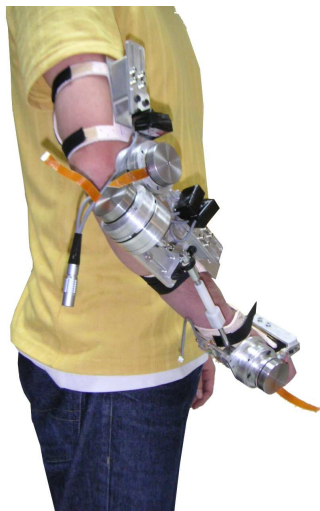
Figure 2: Upper limb robotic exoskeleton. The device spans the human elbow and wrist joints.
