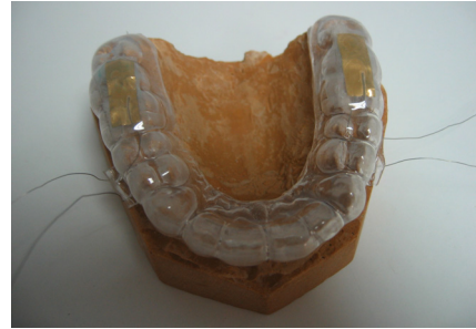
Figure 8: Splint with piezoelectric sensors for diagnosing bruxism.
