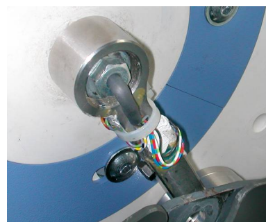
Figure 2: The right crank with the strain gauges wires passes through the axis to be connected to the wireless device that is on the other crank.
