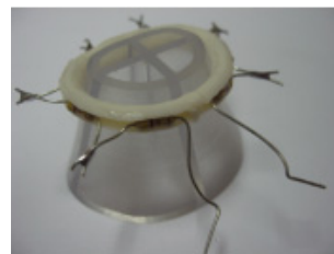
Figure 7: Active ring with heating resistances with the temporary shape already applied. It is ready to be implanted and subsequently activated.
