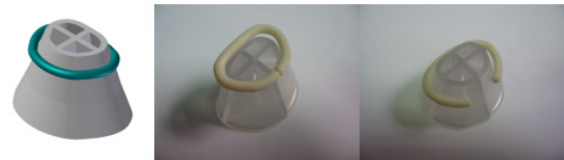
Figure 6: Design and prototype of a tool for programming shape memory effect. Deformation caused at 80 °C to obtain a temporary shape.
