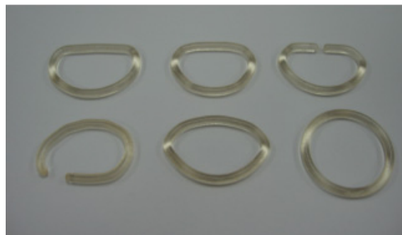
Figure 3: Models obtained by laser stereolithography from files containing the 3D part geometry.
