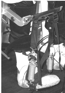
Figure 4: Passive sling of LOKOMAT.
