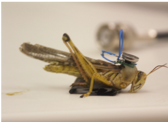
Figure 5: Locust with micro radio installed.
