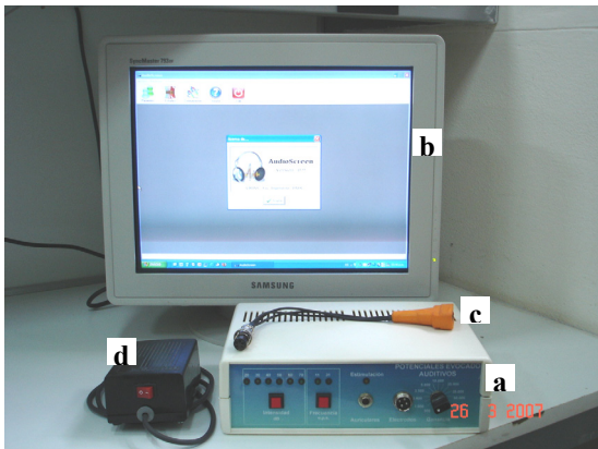
Figure 5: AudioScreen system with the software running on the computer; (a) screener; (b) software interface; (c) electrode cable; (d) power supply.
