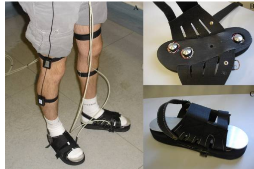
Figure 4: (A) System mounted on healthy individual; (B) Detail of sensor positioning in the sandal; (C) Instrumented sandal.
