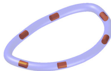
Figure 1: Preliminary active annuloplasty ring design. SMP with internal resistances for heating.
