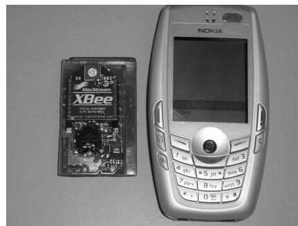
Figure 3: Photo of the sensor node and the smart phone used as the central device.
