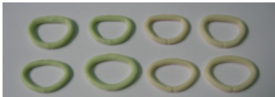
Figure 5: Different polyurethane resin prototypes obtained under vacuum casting in silicone moulds. Both open and closed rings were made to analyse alternative performances.
