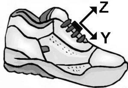
Fig. 1. The accelerometer sensor mounted on a shoe and the acceleration axes orientation.
