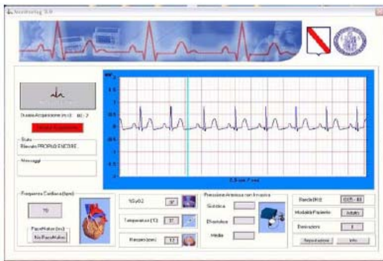
Fig. 2. Software interface for the acquisition of the data from the Patient Monitor Welch Allyn
