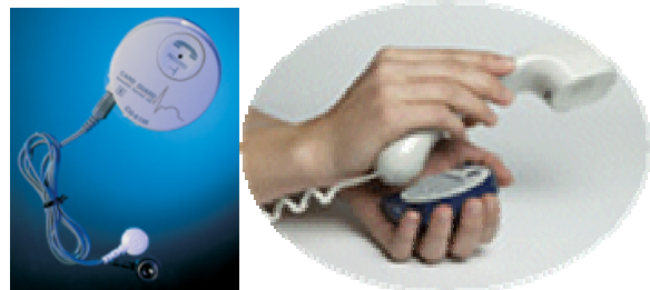
Figure 4: devices for the acquisition and the transmission of the ECG via analogical telephonic line.
