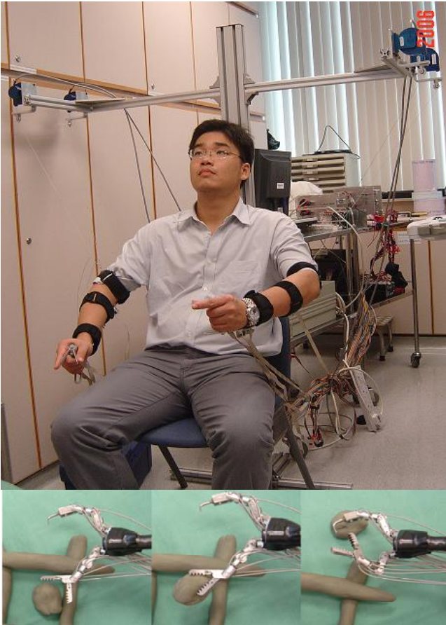
Fig. 8. Using the robotic system for pick and place tasks
