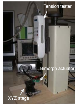
Fig. 5. Photo of Pulling experiment setup
