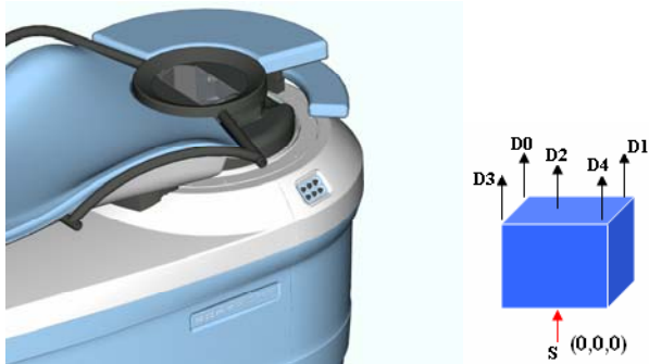
Figure 1: (a) Depiction of the SoftScan™, a time domain multi-wavelength breast imaging clinical device developed by ART Advanced Research Technologies Inc. (b) Source-detector geometry raster-scanned along the periphery of the rectangular slab containing the breast and an optical matching liquid.
