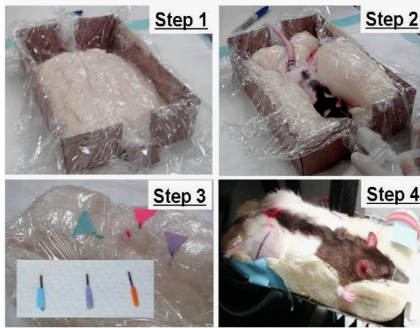
Figure 1. Step-by-step fabrication of animal-specific molds for immobilization and reproducible positioning for imaging of mice or rats.
