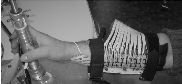
Fig. 1. The depicted 60 channel electrode sleeve is connected via a multiplexer with a current regulated electric stimulator. Muscle selectivity was measured with five strain gauge sensors at each finger digit during electrical stimulation of finger flexor muscles.
