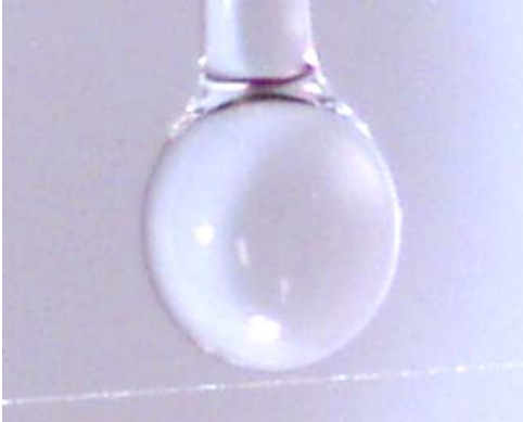
Fig. 4. View of 300 \mu\text{m} silica microresonator and eroded delivery fiber
