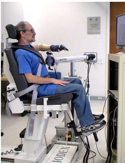
Figure 1. Subject shown sitting in the ACT 3D . He is sitting on the Biodex chair with his arm resting in the splint attached to the HapticMASTER. The computer monitor in front of him shows an avatar of his arm.
