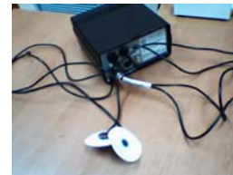
Figure 12: EEG based prototype for monitoring the driver status based on four STFive fuzzy processors
