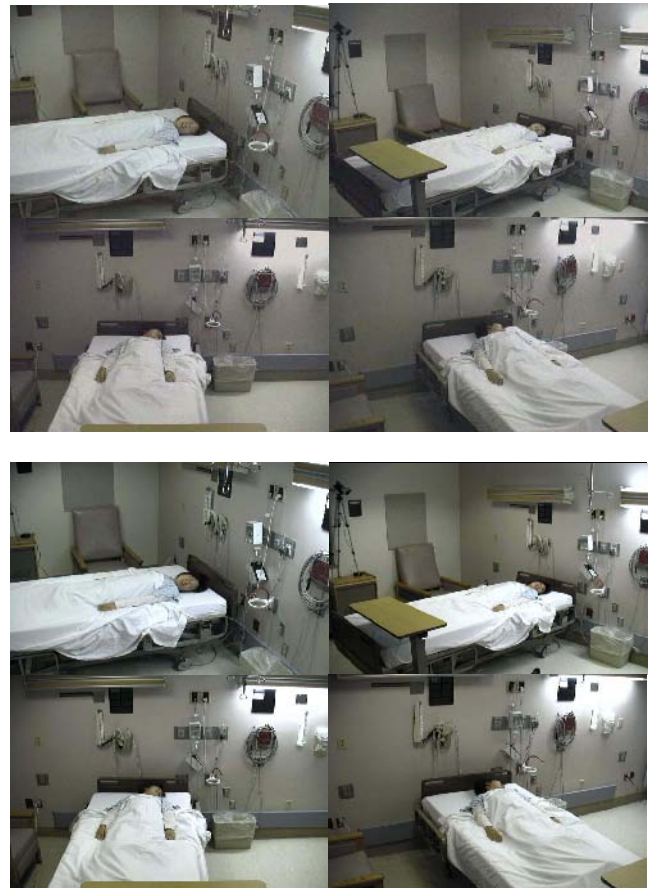
Fig.6. Images reconstruction. The upper four images are the reconstructed image from the synthesized one, where the JPEG codec is used with the q_JPEG value of 65. The bottom four images are those coded separately, with the same q_JPEG value.
