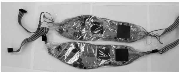
Fig. 1. The underside of the Sixteen Sensor Insole, showing the sizes and locations of the force sensitive resistors. The side showing was placed down next to the insole of the shoe, and the subject's foot made contact with the opposite side of the insole.
