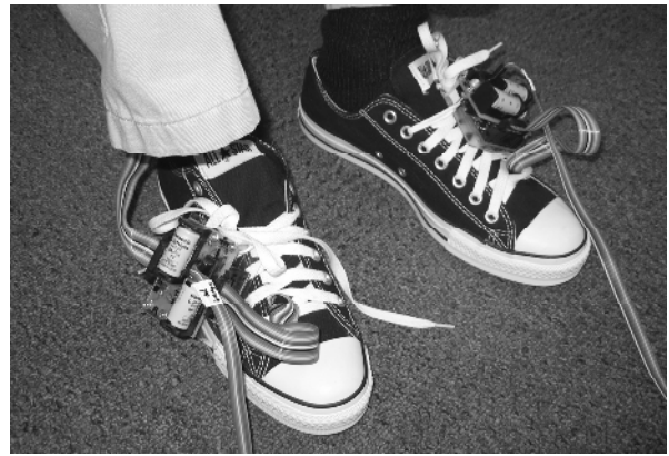
Fig. 2. The circuitry for the Sixteen Sensor Insole, mounted on a sample pair of shoes. The 3 m tether is connected to a DAQ board and a computer for control of the multiplexers and data acquisition.
