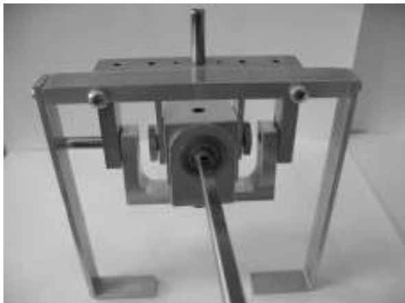
Fig. 1. Gimbal setup serves as the fulcrum point at the cervical canal allowing 4-degrees of movement.
