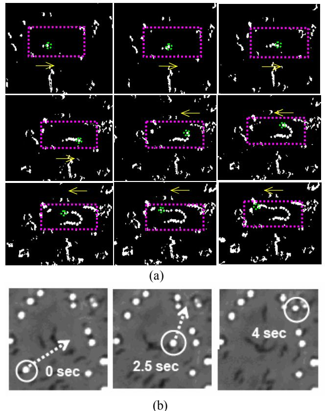
Fig. 6. a) A *MC-1* bacterium is pushing a fluorescent microsphere ( $2\mu\text{m}$  in diameter) to execute a U-turn when reverse the magnetic field (12Gauss). b) A *Magnetospirillum gryphiswaldense* bacterium is pushing a microsphere ( $3\mu\text{m}$  in diameter) to the north pole of an electromagnet (100 Gauss)
