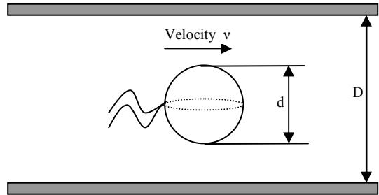
Fig. 4. According to Eq. 3, with a fluidic channel (diameter of  $10 \mu\text{m}$ ) and a velocity of the *MC-1* bacteria of  $200 \mu\text{m/s}$  in unbounded conditions, the velocity of the bacteria will be decreased to approximately  $120 \mu\text{m/s}$  due to the wall effect.
