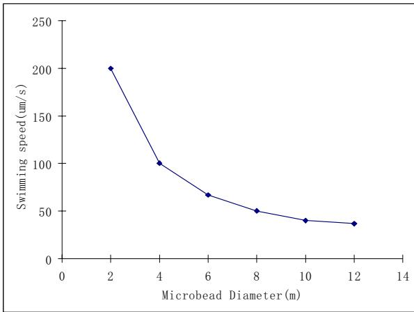
Fig. 5. Velocity of a microbead being pushed by a single MTB for various bead diameters, assuming that the swimming speed of MTB is  $200\mu\text{m/s}$  before being attached to the microbead.
