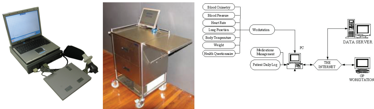
Fig. 1. Redesigned TeleMedCare System showing (left panel) the client workstation with laptop and clinical measurement modules (single lead ECG, blood pressure, spirometry, pulse oximetry, temperature, Bluetooth-enabled weight scale (not shown)). The middle panel shows the system mounted on a medication trolley with touch screen and biometric finger print reader for authentication and medication authorization. The right panel is a schematic of the system illustrating the client-side functionality and the clinician access (for management and reporting functions) via a standard Web browser.
