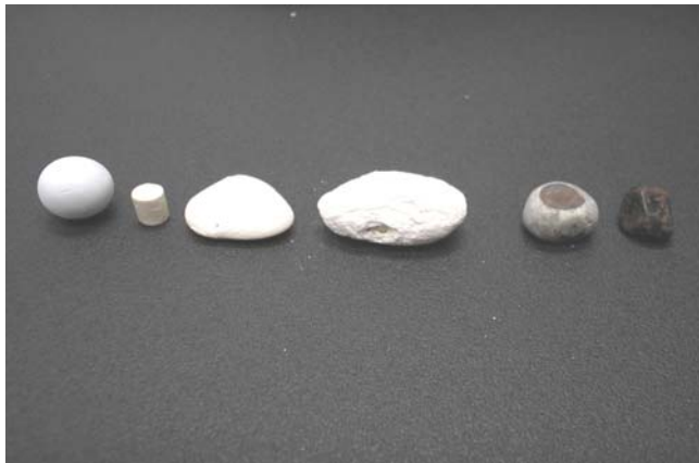
Fig. 2. Phantoms and different composition renal calculi are shown. From left to right are HMT spherical phantom, U-30 cylindrical phantom, calcium carbonate-magnesium-xantine real renal calculi, calcium carbonate-magnesium-amonia-colesterol renal calculi, only calcium carbonate renal calculi, phosphate-calcium carbonate-amonia renal calculi.
