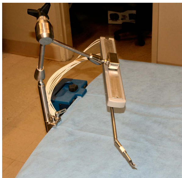
Fig. 1. New robotic instrument design with articulated elbow joint inside patient body cavity
