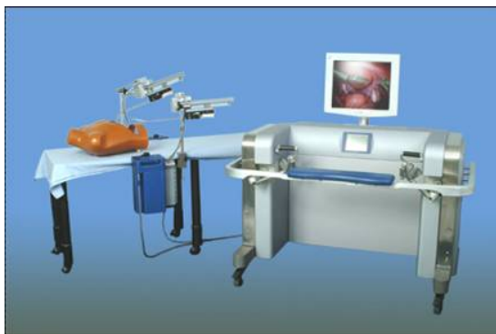
Fig. 3. Laprotek system with instruments mounted to OR table.
