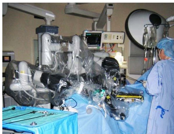
Fig. 2. The daVinci system during an actual urology procedure. Access to the patient is severely limited by the mechanism in the sterile field over the patient.
