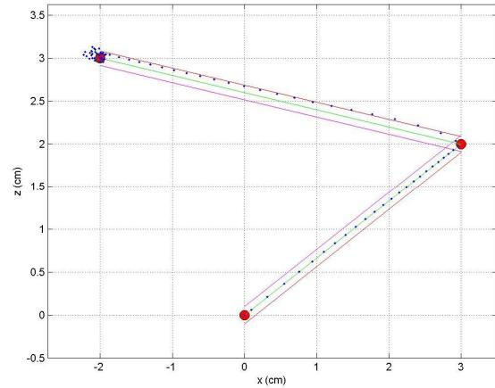
Fig. 6. Plots of the 2D simulated trajectory along the x and z axes of a chrome steel bead of 1.5 mm in diameter along a horizontal duct of 3 mm in width, with  $v_f = 5$  cm/s with acquired with a PID controller whose gains are with  $K_{TP} = 0.4$ ,  $K_{TD} = 0.2$ ,  $K_{TI} = 0.2$ ,  $K_{NP} = -3$ ,  $K_{ND} = 0.2$ , where the final waypoint coordinates are  $x = -2$  cm and  $z = 3$  cm, and the intermediate waypoint coordinates are  $x = 3$  cm and  $z = 2$  cm.
