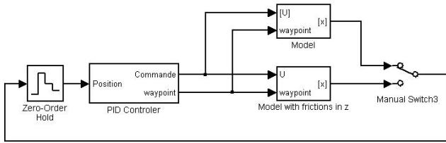
Fig. 3. Block diagram of the discrete closed loop control system
