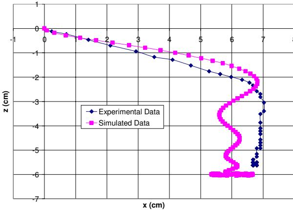
Fig. 4. Plots of the 2D experimental and simulated trajectory of a chrome steel bead of 1.5 mm in diameter along a horizontal plane, in a quiescent flow acquired with a PID controller with  $K_{TP} = 0.4$ ,  $K_{TD} = 0.2$ ,  $K_{TI} = 0.2$ ,  $K_{NP} = 0$ ,  $K_{ND} = 0$ , where the target coordinates are  $x = 6$  cm and  $z = -6$  cm.
