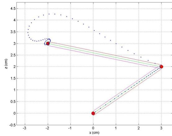
Fig. 5. Plots of the 2D simulated trajectory along the x and z axes of a chrome steel bead of 1.5 mm in diameter along a horizontal duct of 3 mm in width with  $v_f = 5$  cm/s, acquired with a PID controller whose gains are with  $K_{TP} = 0.4$ ,  $K_{TD} = 0.2$ ,  $K_{TI} = 0.2$ ,  $K_{NP} = 0$ ,  $K_{ND} = 0$ , where the destination coordinates are  $x = -2$  cm and  $z = 3$  cm, and the intermediate waypoint coordinates are  $x = 3$  cm and  $z = 2$  cm.
