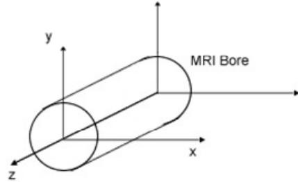
Fig. 1. Axis convention in the MRI environment.
