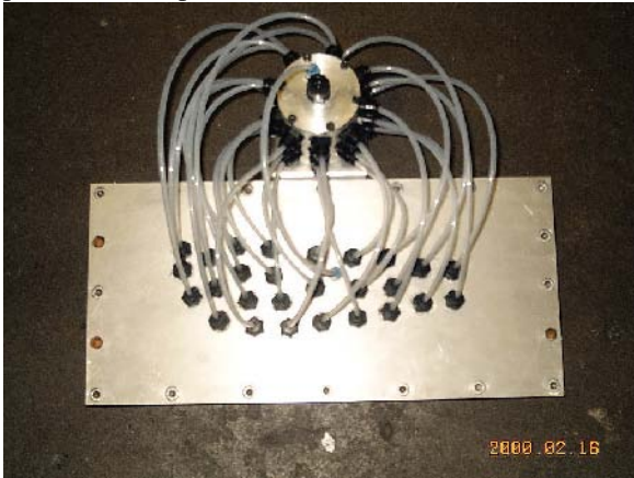
Figure 2: The pressure vessel was designed with 28 airlines for uniform redistribution of compressure air inside the vessel.
