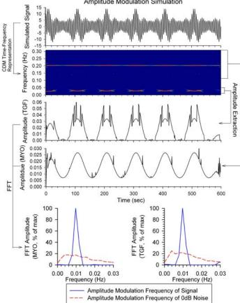
Figure 1 – Extraction of amplitude modulation from a simulated signal. The simulated signal contains two frequencies (0.03 and 0.2Hz) modulated by a low frequency (0.01Hz).
