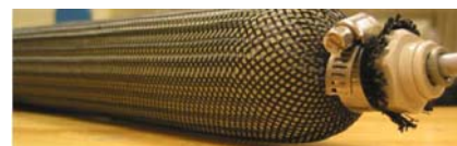
Fig. 1. Pneumatic muscle actuator (Mckibben Muscle) made in lab.
