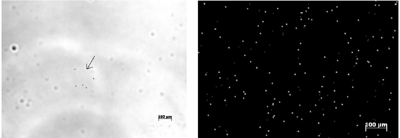
Fig. 4. BF and DF simulated images containing respectively 5 and 200 bacteria agglomerations.
