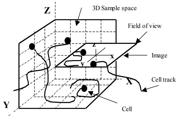
Fig. 2. The intermediate ideal image is the intersection between the camera field of view and the cell geometries at time  $T$ . (Figure is not to scale.)
