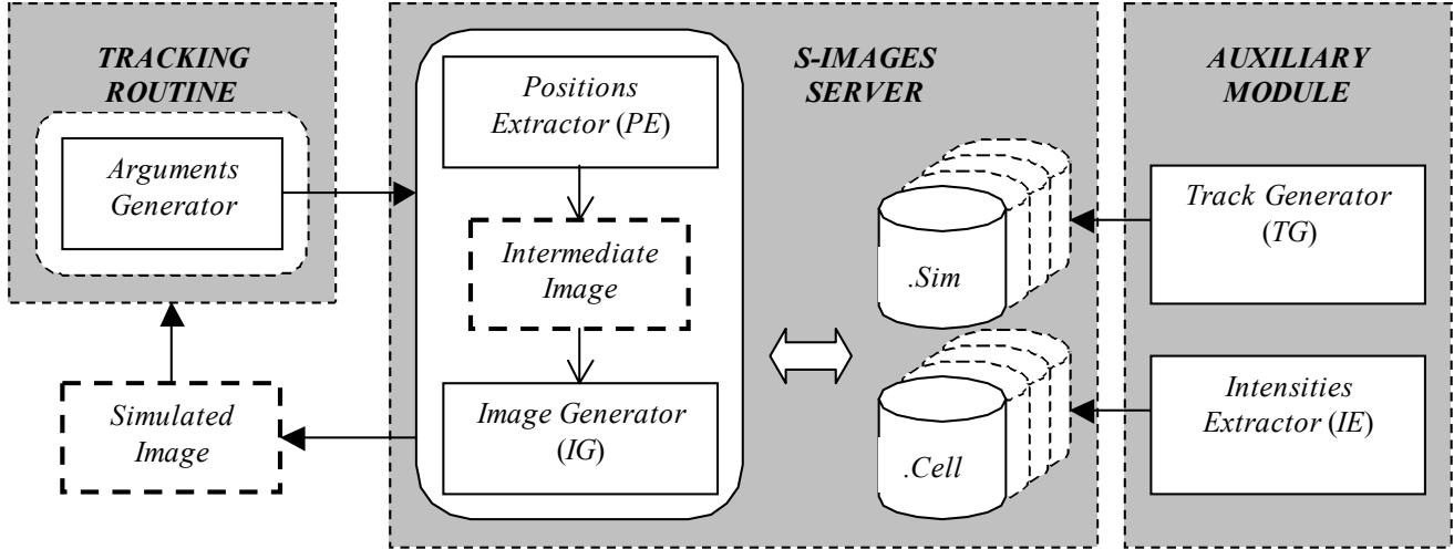
Fig. 1. The architecture of the simulation system. During one cycle, the tracking routine sends a request to the *SIS* with the following arguments: time  $T$ , stage position and a *simulation*, and receives a simulated image back, at the expense of a minor modification in the image acquisition module.
