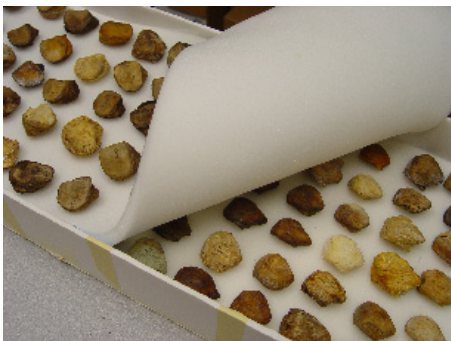
Figure 1: In vitro patellae prepared for CT scanning
