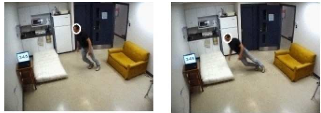
Fig. 1. Head position (localized with an ellipse) during a fall on two successive images. In this case, the movement is about 70 pixels at 30Hz and image with size 640x480.
