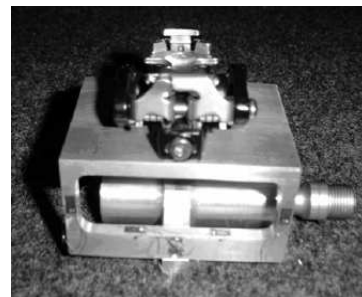
Figure 1 : pedal prototype with strain gauges.
