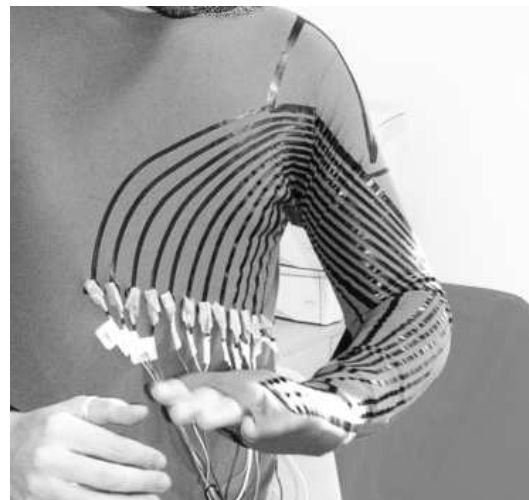
Fig. 1. Sensing stripes (thick line) and connecting wires (thin) are CE elastomer printed on fabric. This is an early, wired prototype.
