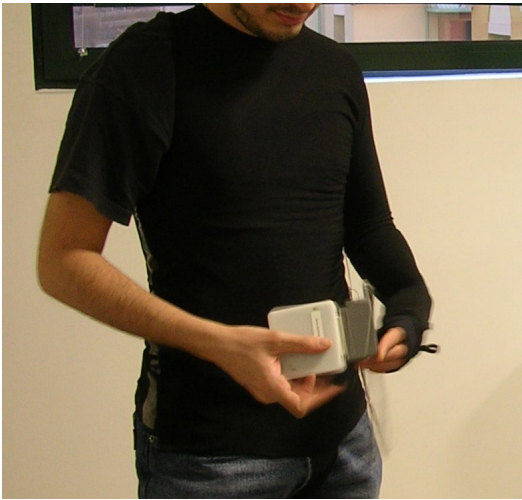
Fig. 2. Current garment prototype, with wireless data acquisition electronics. Printed strain sensors are invisible because placed between two layers of Lycra.
