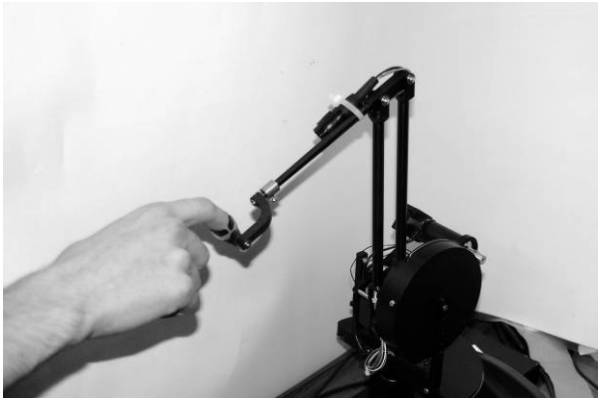
Fig. 1. The SensAble PHANTOM Premium 1.5 haptic interface was used for the experiments in this study.
