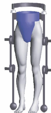
Fig. 1. A schematic drawing of the gait support system for human locomotion. There are two degrees of movement, at the hip and knee, on each assistance leg. The support system and the operator have a rigid connection at the pelvis only, not through the legs.
