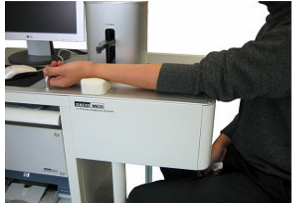
Fig. 3. Pulse pressure of radial artery measurement by 3-D MAC
