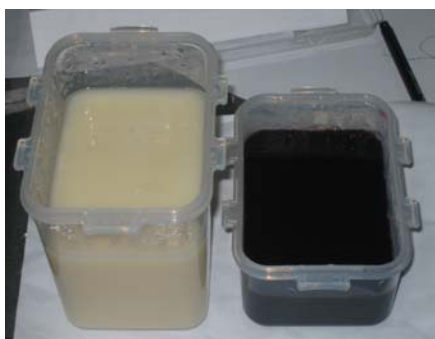
Fig. 2. The Photograph of fabricated fat (left) and muscle (right) phantoms.
