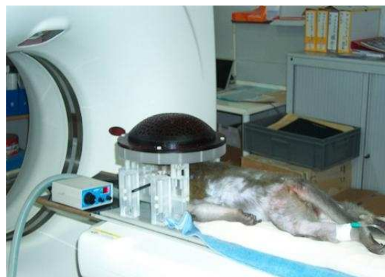
Fig. 4 Monkey in the CT scan with its stereotactic frame. The front part of the therapy probe has been put on the frame in order to locate the position of each transducer.
