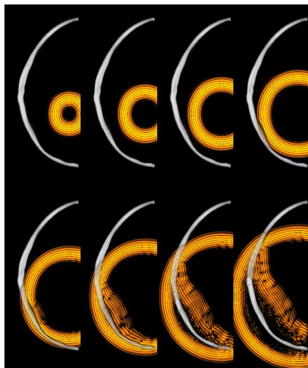
Fig. 6 Propagation from virtual source point through skull bone using finite difference code.
