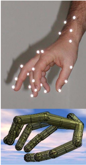
Fig. 1. (top) Snapshot of a hand instrumented with reflective markers for optical motion capture. (bottom) Our physically simulated hand attempting to achieve the captured hand configuration above.
