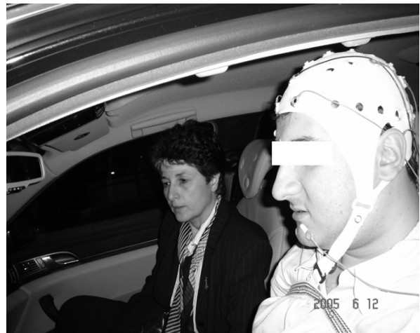
Fig. 1. The subject No. 1 in front of the wheel wearing the EEG cap before the experimental procedure. The driving instructor was seated next to the driver.
